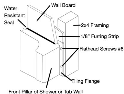
4. Attach the bathtub with screws to each stud. Use screws that are long enough to penetrate the studs if installing over previously installed drywall, or into a firewall pocket installation.
